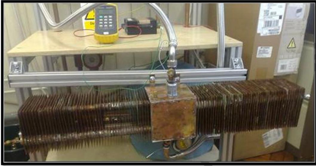
**Figure 6:** Heat pipe radiator prototype
