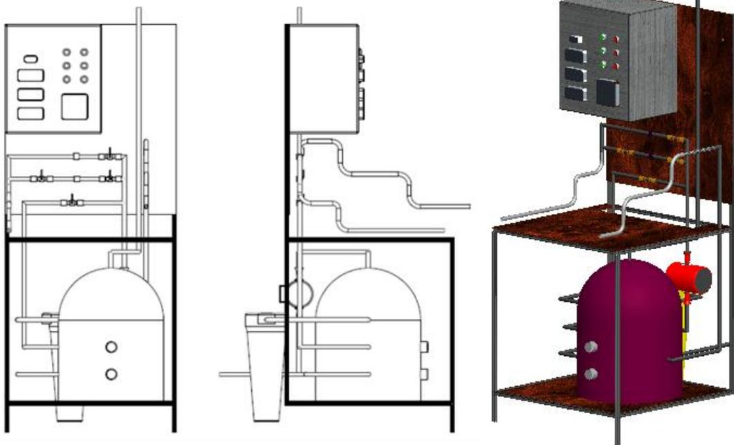
**Figure 7:** (Top) Schematic of thermal performance characterization test facility. (Bottom) CAD renders of the test facility.
