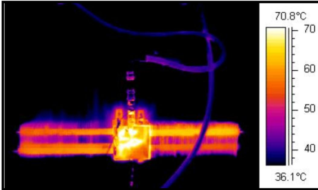
**Figure 8:** Thermal image of heat pipe prototype radiator.
