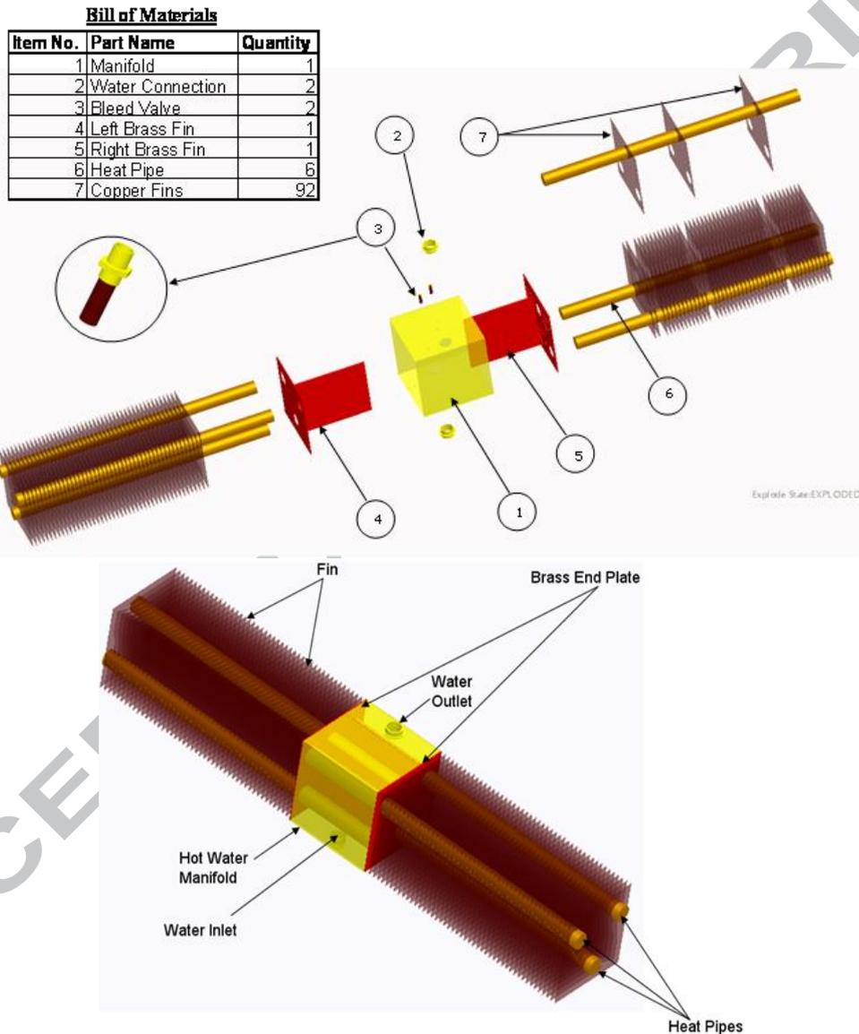
**Figure 1:** Schematic of double convector heat pipe-based heat exchanger (top) assembly drawing (bottom) assembled unit.
