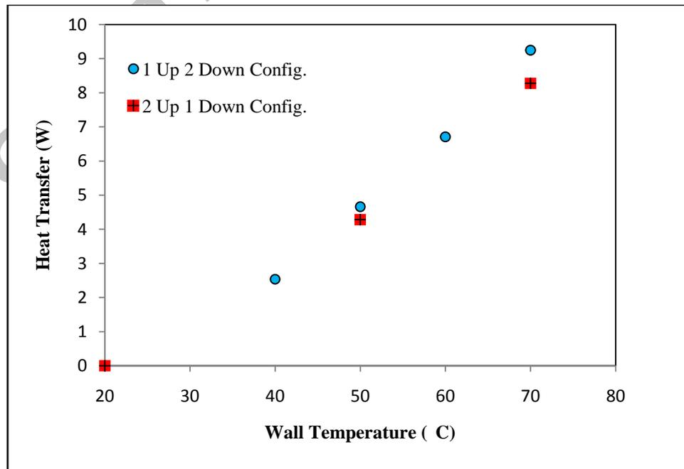
**Figure 5:** Heat transfer rate versus heat pipe wall temperature for a single channel for ambient temperature of 20°C.
