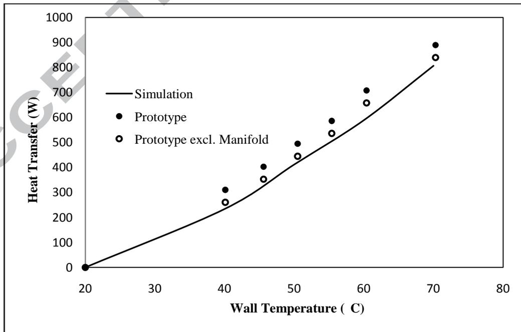
**Figure 9:** Power output versus water inlet temperature / wall temperature comparing experimental prototype with simulations for ambient temperature of 20°C.
