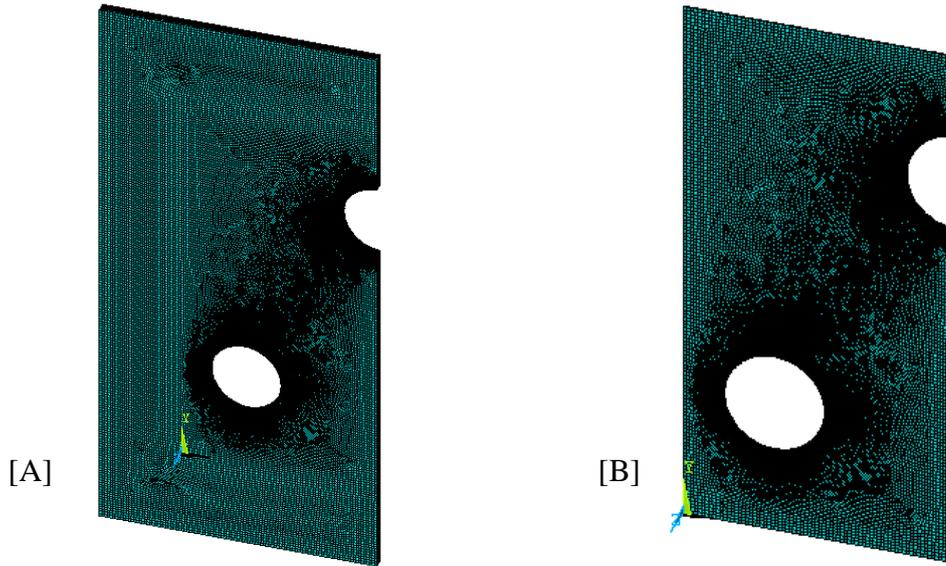
**Figure 2:** Example of the meshed elemental structure for both the [A] air and [B] fin models.
