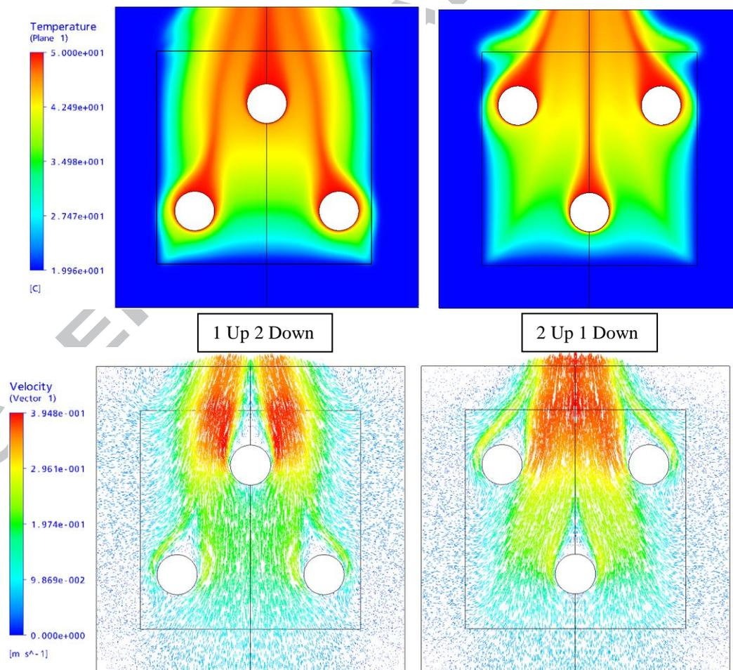
**Figure 4:** Simulations for 50°C heat pipe wall temperature. *Top:* the temperature profile through the centre of the air channel of both 1 up 2 down and 2 up 1 down tube configurations. *Bottom:* Vector plot of the velocity of the air in the centre of the channel.
