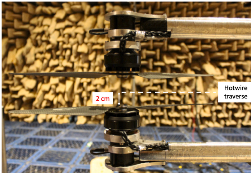
Fig. 12. Photograph of overlapping rig inside the ISVR anechoic chamber.
