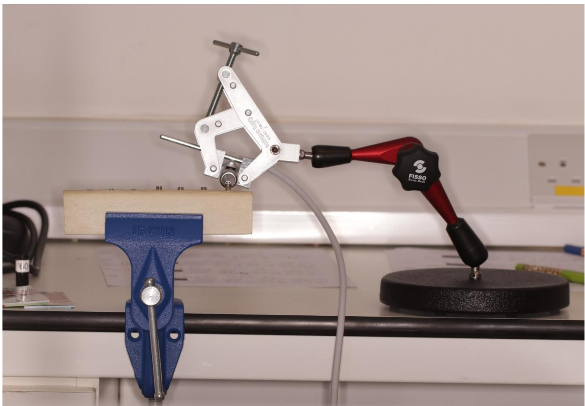
Figure 21: Experiment Set up: Fisso Articulated Arm holding the Periotest™ handpiece at the correct distance to enable measurement of the stability of the individual implants placed in the synthetic bone block that is immobilised in the vice.
