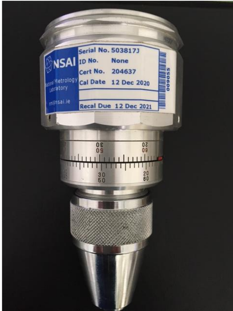
Figure 17: Calibrated torque wrench ((Tohnichi®.)
