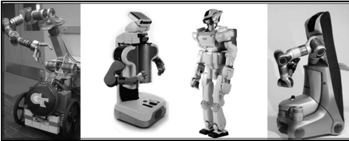
Figure 1: from left to right: Golem-Krang, the PR-2 robot, HRP-C, the Care-O-Bot robot
