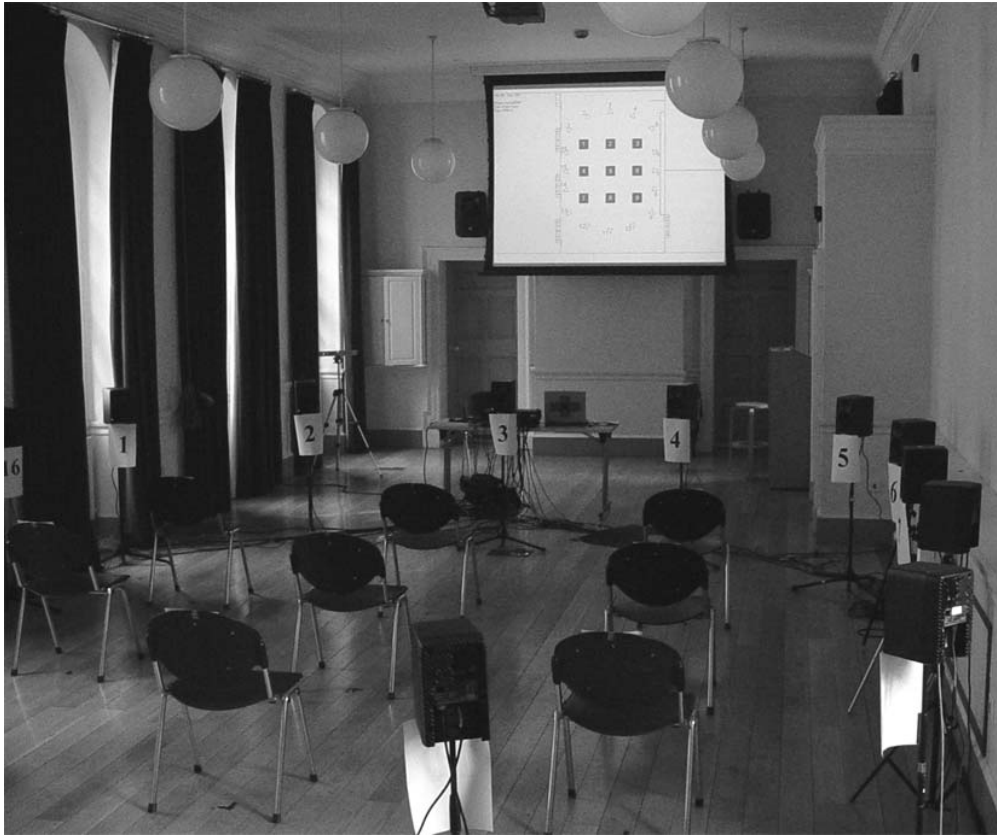
Fig. 6.7 Listening tests loudspeaker configuration
