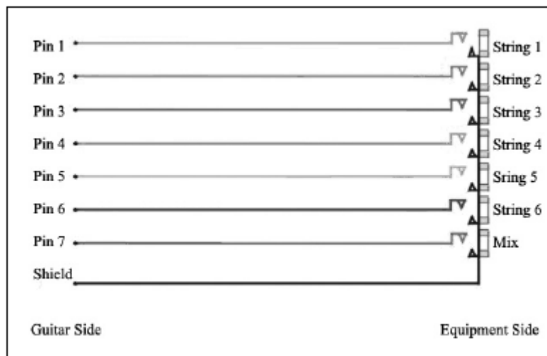
Fig. 11.4 13-pin breakout box schematic
