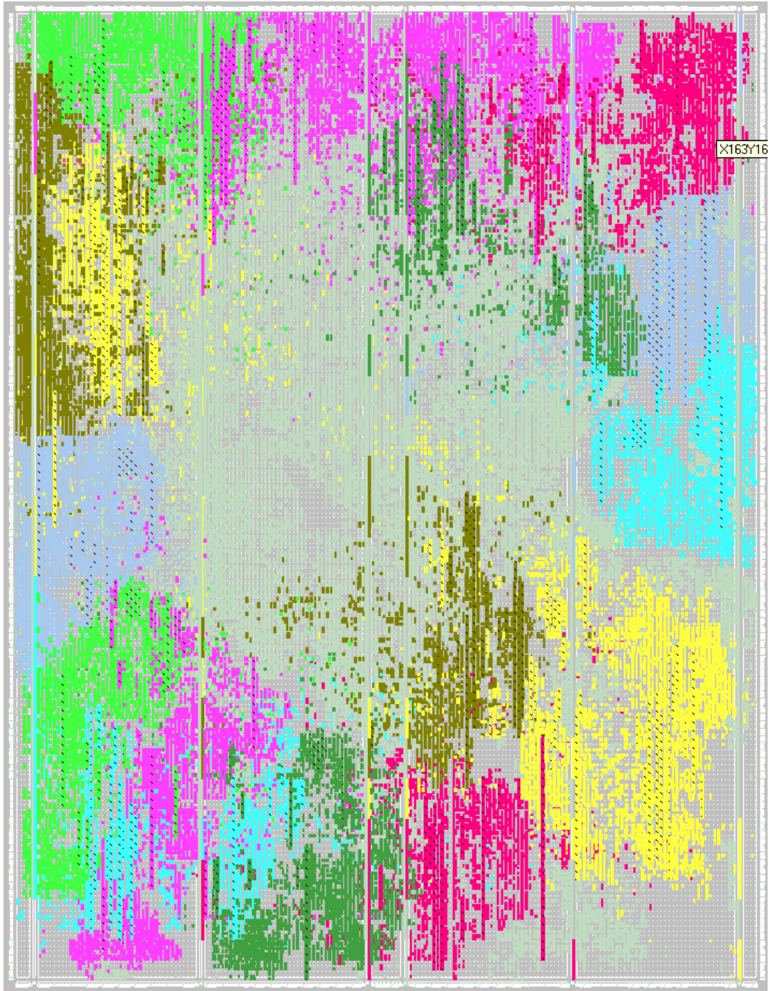
Figure 9-a. Layout of FPGA when programmed with the double precision Dirac operator design from Chapter 6. Each of the blocks of colour is one of the arithmetic units, the light green colour is the general application logic. Any grey areas represent logic that is not used in the design.
