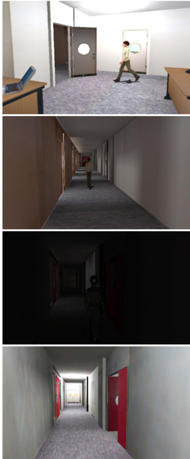
Figure E.1: 1) An occupant finishes work and leaves the office. 2) The occupant enters corridor to move to another location. 3) The lights have been switched off and the corridor is in darkness. 4) The occupant activates the motion sensor in the stairwell and the lights switch on but the occupant is not longer present.
