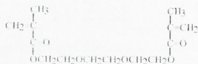
Figure 3.1: The chemical structure of (a) bisphenol A glycol dimethacrylate (Bis-GMA) and (b) triethyleneglycol dimethacrylate (TEGDMA) utilised in the monomer blend of the dimethacrylate RBC, Z100™.
