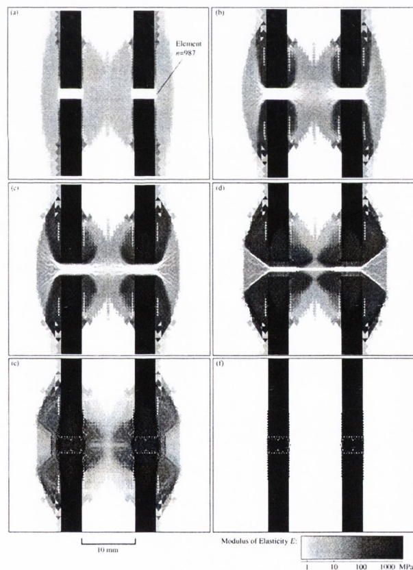
Figure 2.19. Predicted modulus of elasticity at (a) day 3, (b) day 14, (c) day 21, (e) day 84, and (f) day 365. After Ament and Hofer [20].
