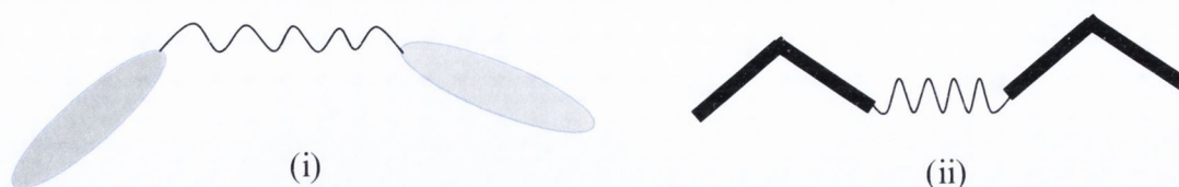
Figure 1.7: Schematic representation of bimesogens composed of (i) rod + rod and (ii) bent-core + bent-core molecules.
