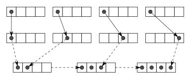
(a) Algorithm 1. Nonconsecutive read of the form a[4 \* i] with VF = 4. First we permute the load-mapped register set so that selected lanes will not collide under vertical composition with blend. We then blend the permuted registers together to form the packed vector corresponding to the access.
