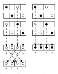
Figure 3-5: Algorithm 5. Our transformation enables vertical composition with the blend instruction of colliding memory accesses with a single transformation of the mapped register set. One access is out-of-order under vertical composition with blend after data layout transformation (left side). However, the vectorization can be legalized with a single permute as shown, to ensure the order of elements in each register is the same.
