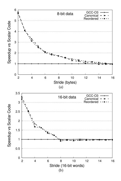
Figure 3-13: Synthetic benchmark results: 8-bit and 16-bit scattering operations
