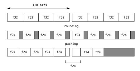
Figure 4-4: Layout of data in **SSE** vector registers before format conversion (top), after rounding to the desired size (center) and the desired layout in memory (bottom).
