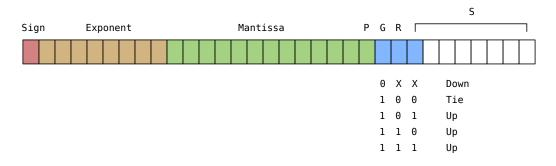
Figure 4-5: Rounding to nearest even. Marked bit positions correspond to Preguard, Guard, Round, and Sticky bits.
