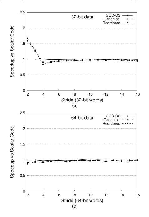
Figure 3-14: Synthetic benchmark results: 32-bit and 64-bit scattering operations
