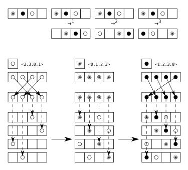
Figure 3-6: Algorithm 6. Accesses a[4 \* i + 2] (light dots), a[4 \* i] (patterned dots), and a[4 \* i + 1] (black dots). Desired store order at top with rotated store order underneath. Required permutation of each access to obtain rotated store order indicated with permute masks. Heavy arrows at bottom show the evolution of the store-mapped register set as each access is interleaved in. Final store-mapped register set before inverse rotation is shown at bottom right.
