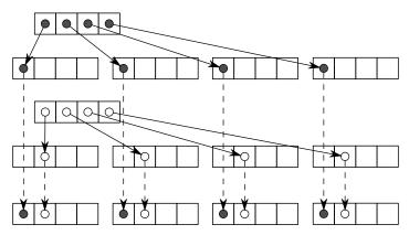
(b) Algorithm 2. Two nonconsecutive writes of the form a[4 \* i] (dark dots) and a[4 \* i + 1] (light dots) with VF = 4 are composed into a single store-mapped register set, reducing the number of stores required.
