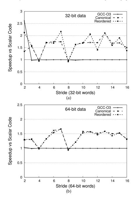
Figure 3-12: Synthetic benchmark results: 32-bit and 64-bit gathering operations
