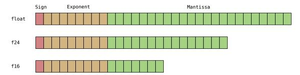
Figure 4-2: Layout of alternative multibyte floating point formats
