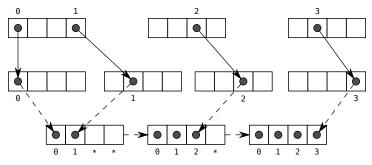
(a) Algorithm 1. Memory access of the form a[3 \* i] with VF = 4. \* denotes a don't-care element in an output register. Elements are labelled with their index in original program order.
