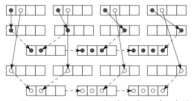
(a) Algorithm 1. Two nonconsecutive reads of the form a[4 \* i] (dark dots) and a[4 \* i + 1] (light dots) with VF = 4, with shared spatial locality can be serviced from the same load-mapped register set using permute and blend sequences.
