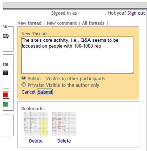
Figure 34: A comment with two attached bookmarks. Each bookmark has annotations added by a user. Clicking the bookmark will load the visualisation, coupled with the annotations, into the interactive Java applet.
