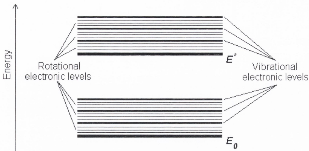
Figure 2-10: Energy level diagram. E_0 represents the ground state while E^* is the excited state.
