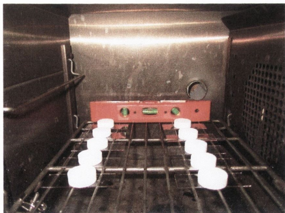
Figure 3-2: Experimental setup for drop casting on teflon disks.
