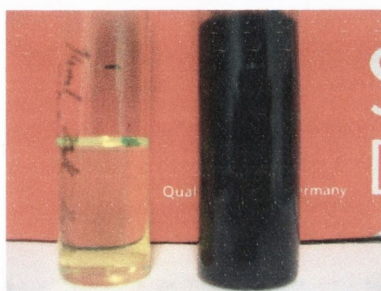
Figure 3-1: Vials of PmPV (left) and nanotube composite (right) in a toluene solution.
