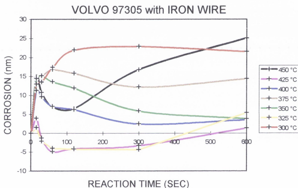
Figure 6.7 Corrosion of iron wire reacted with Volvo 97305
