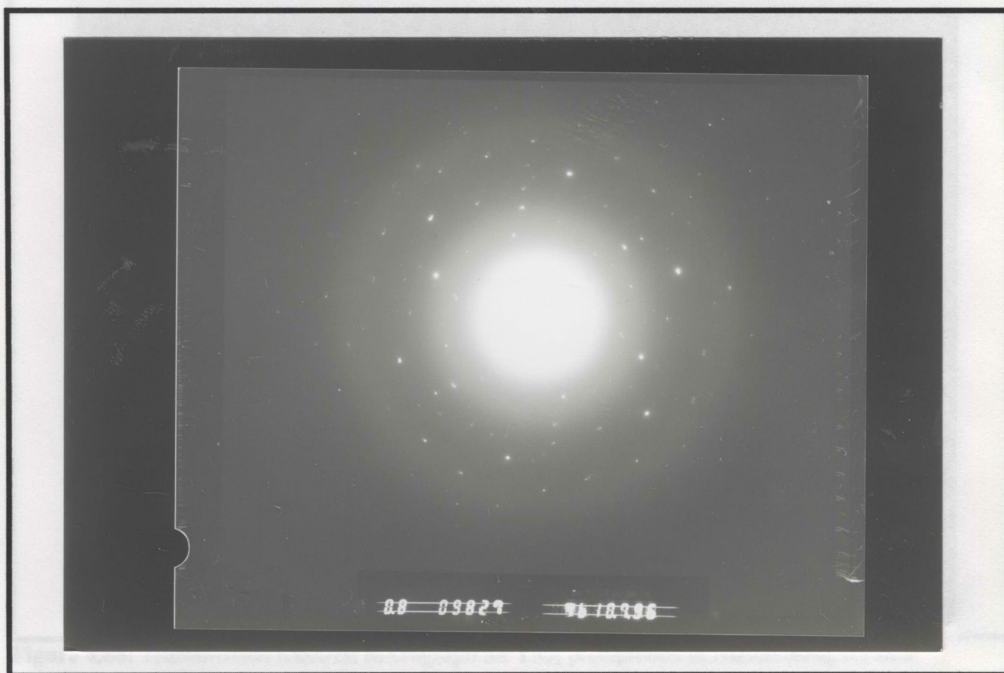
Figure 4.64: Electron diffraction pattern for Cd-St (130 layers) deposited on Quartz. Camera length = 0.8 m \lambda_{el.} = 0.0037 nm
