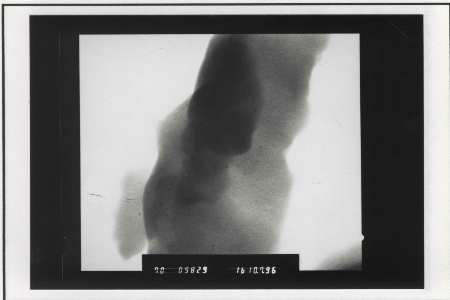
Figure 4.63: Transmission Electron Micrograph for Cd-St (130 layers) deposited on quartz.
