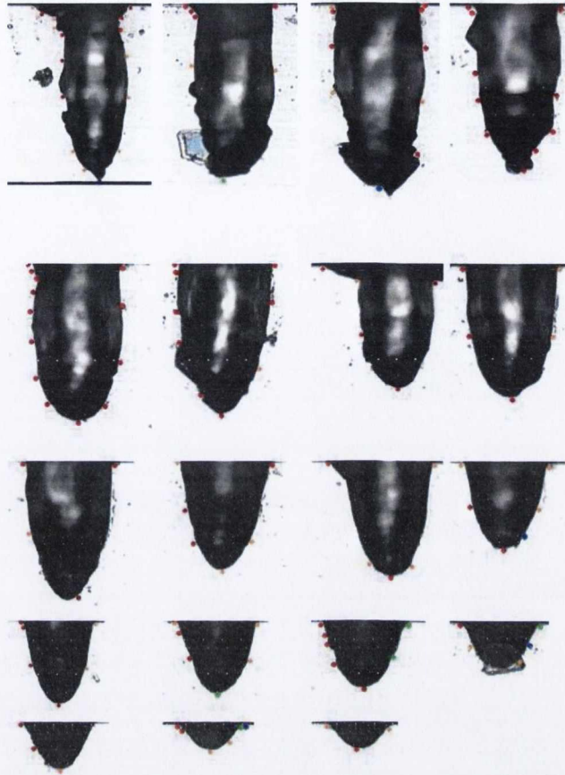
Figure 4.13 – Sample s4, \varnothing=50\mu\text{m} , singlestep: primarily tensile stress uniform along sidewalls and generally less than 150MPa.
