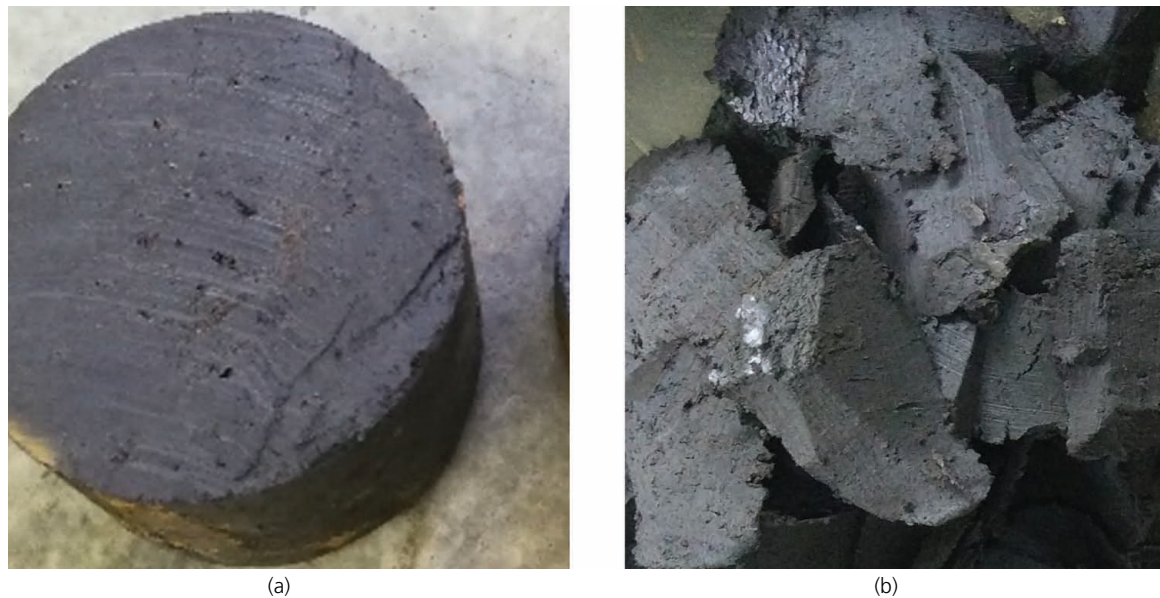
Figure 2. Sampled largely amorphous peaty soils retrieved from 8.4 m depth at the Dian-Chi Lake area using the sampler shown in Figure 1: (a) recovered core ( w_n = 142\% , N = 23.5\% ); (b) sample trimmings ( w_n = 192\% , N = 34.8\% )
