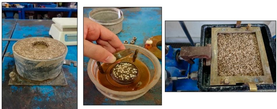
Figure 5. CBR (left), oedometer (centre), and shearbox (right) soil–EPS beads test-specimens.
