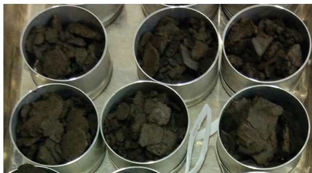
Figure 2. Wet specimens prepared for the oven-drying tests. Note that the specimen tins are resting on the lids used to cover them during the cooling periods in the desiccator
