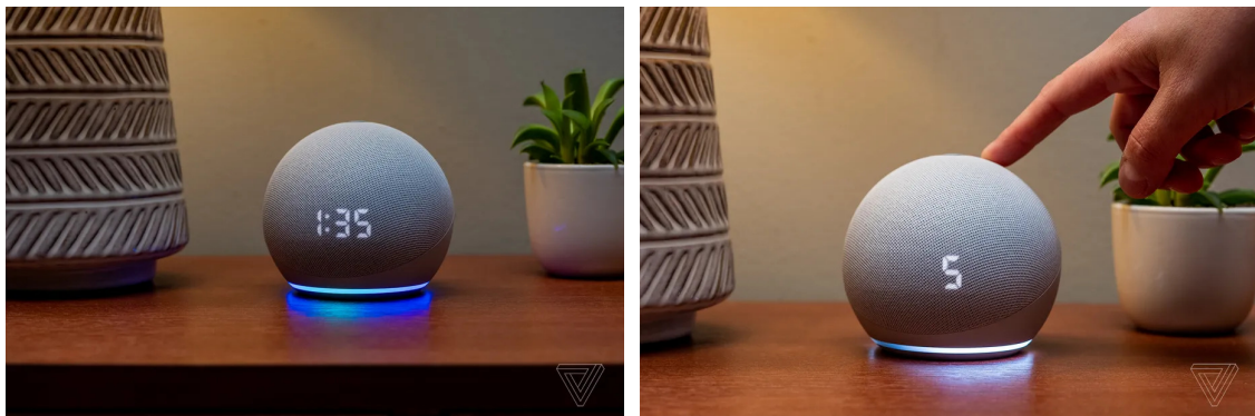
Figure 4.3: The Amazon Echo supports both voice control and touch input. An accessible price point, useful functionality, and appealing design have made such touchless devices common. ©The Verge 2020.
