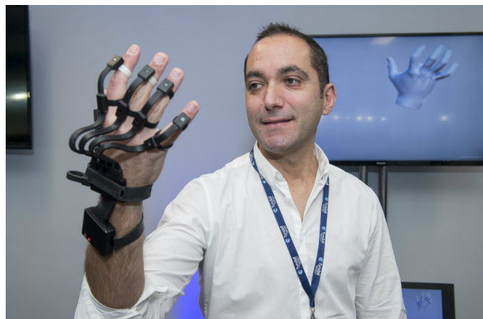
Figure 4.5: Tyndall’s Smart Glove provides an easy-to-wear solution that can allow the user to interact with both digital and physical devices [125] . Reproduced with permission.
