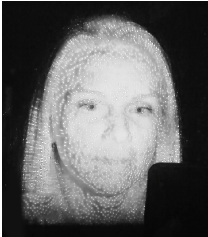
Figure 4.4: Apple Face ID authentication functions by projecting and analysing thousands of IR dots to create a depth map of the user's face sensors. ©iFixit 2017. Reproduced with permission.
