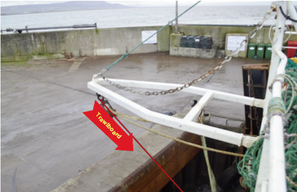
Appendix 7.15 Photograph No. 7 - A Frame
