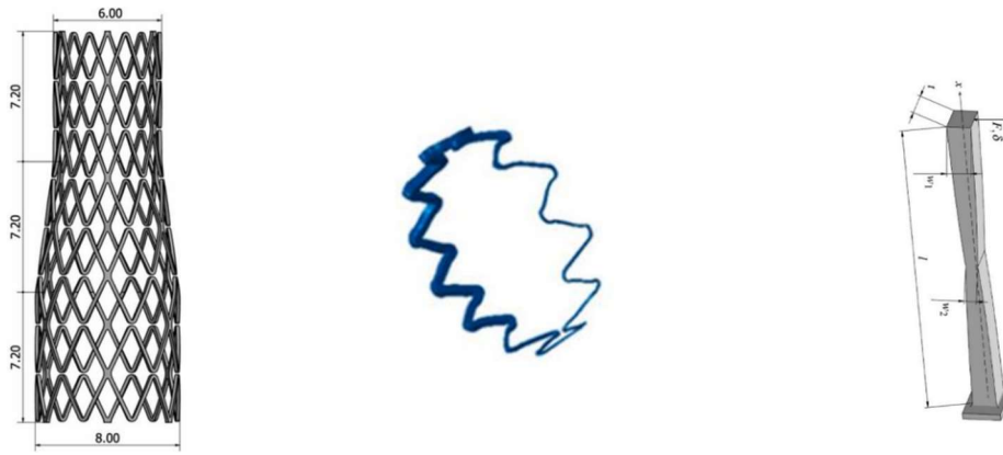
Figure 66 Examples varied diameter, varied thickness, and tapered strut profile stents [9], [10],[11]
