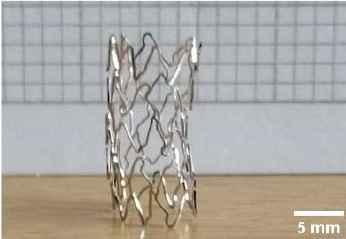
Figure 60 BARD Valeo vascular stent after compression testing
