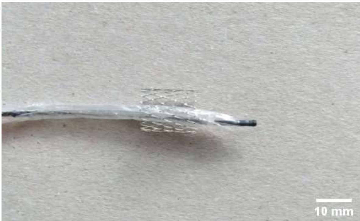
Figure 44 AM IntraStent placed on 2 mm diameter Boston Scientific Express LD stent delivery system.
