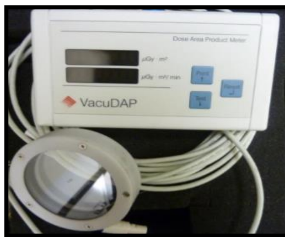
FIGURE 2.3 DAP meter used to obtain DAP values at the exit of the X-ray beam.
