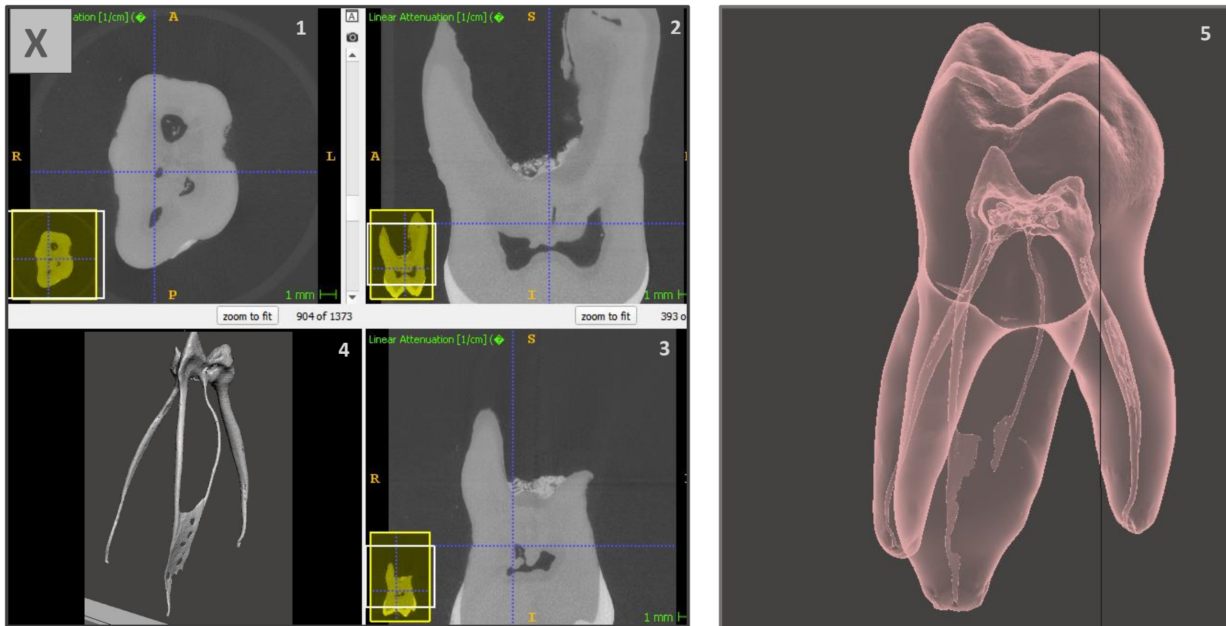
FIGURE 4.1a Tooth X: MicroCT images reconstructed in ITK-SNAP from DICOM files ( 1-3 ). Segmented meshes reconstructed in Meshmixer from STL files of the pulp chamber and root canal anatomy ( 4 ) and the entire hard tooth structure using toggle visibility ( 5 ). ITK-SNAP: software application used to segment structures in 3D medical image. DICOM: Digital Imaging and Communications in Medicine.
