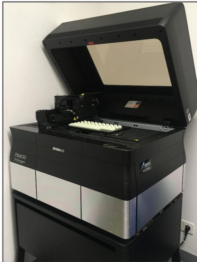
FIGURE 4.4 Laserjet printer used to print 3D teeth: Objet 30Prime (Stratasys Ltd, Minneapolis, MN, used for printing M1M's (Würzburg Dental Hospital, Germany). M1M: First Maxillary Molar.
