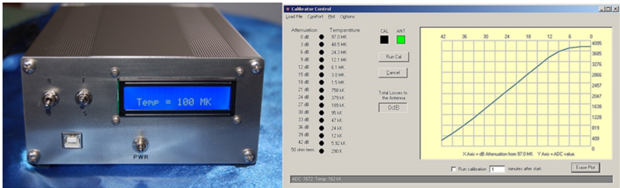
Figure 4: Automatic multistep calibrator and the RSS software calibrator control panel showing the response of an SDRplay RSP1A receiver.
