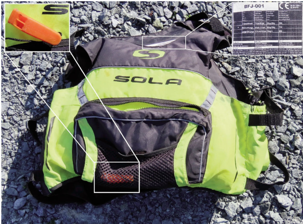
Figure 5: The type of buoyancy aid used by the kayaking group, highlighting the provision of a whistle and this product's compliance with the European Standard for PFDs, EN ISO 12402-5.
