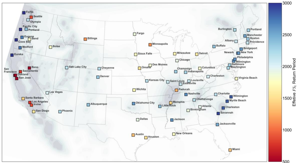
Figure 5: Average effective design FS_L return period for an example soil profile using current ASCE 7 design procedures and ground motions, computed from PLHA-based liquefaction hazard curves. Data overlaid on greyscale contour map showing relative seismic hazard from the USGS 2018 NSHM.
