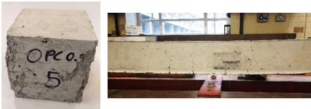
Figure 4: Test specimens used in this study (a) concrete cube (b) concrete beam
