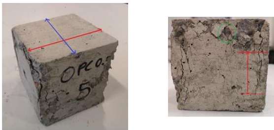
Figure 8: (a) Calibrating the concrete cube dimensions (b) Crack measurements
