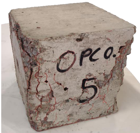
Figure 5: Concrete cube 3D model with crack locations marked on the model
