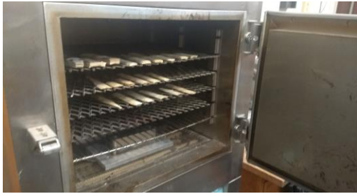
Figure 1: Setup for moisture content tests.
