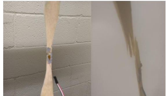
Figure 5: Failure in tension test specimens.
