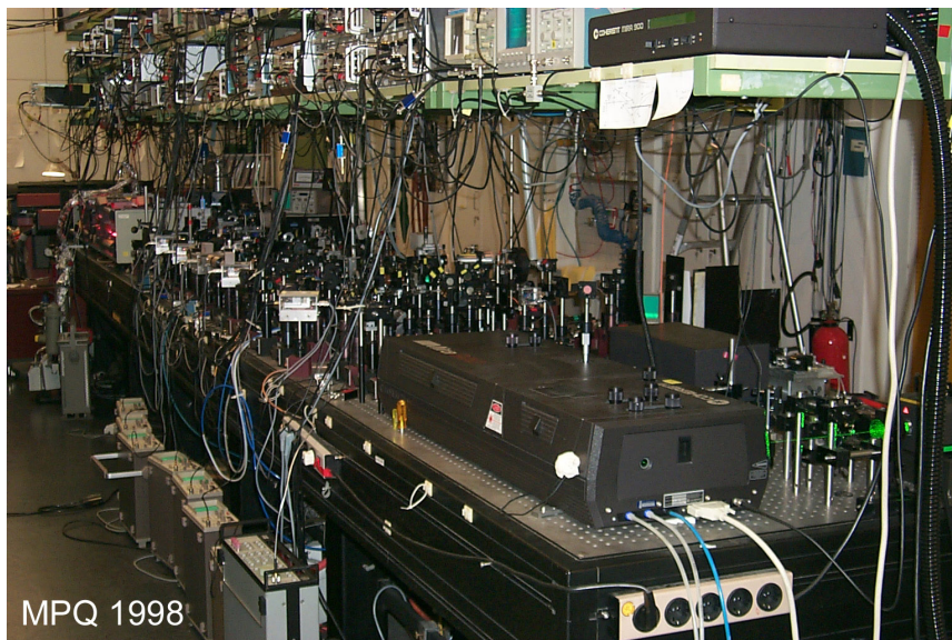
FIGURE 1.3: The first self-referenced optical frequency comb at the Max-Planck Institute for Quantum Optics in 1998.
