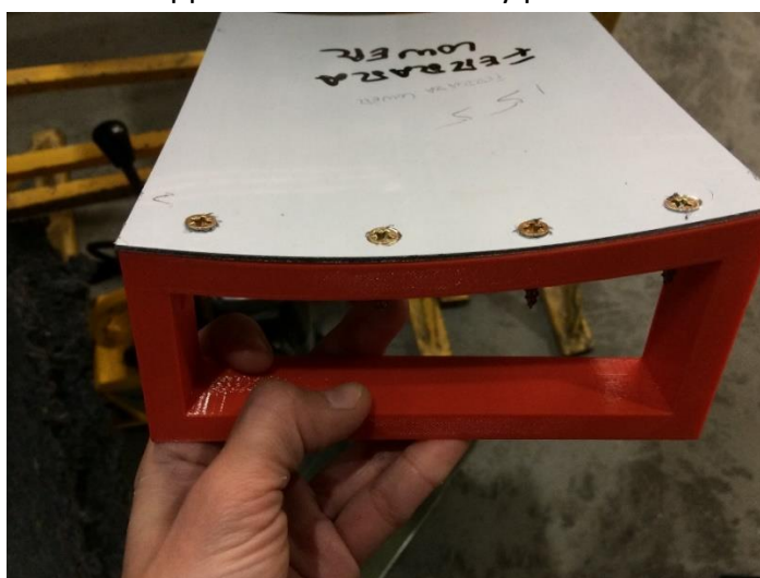
Figure 5. 9 Auxiliary plates installed on the reflector support
