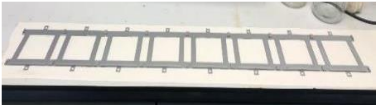
Figure 6. 6 Full string of eight solar cells holders
