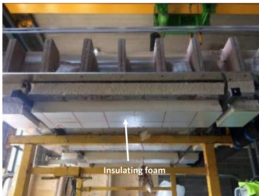
Figure 6. 21 Insulation installed in the PCM containers
