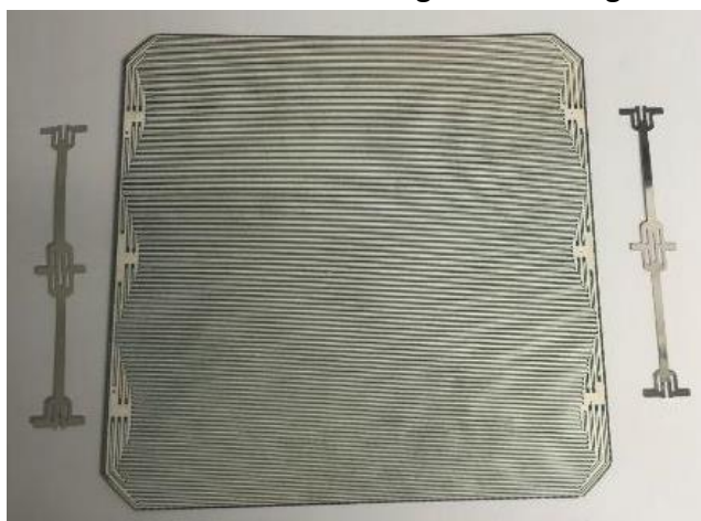
Figure 3. 10 Back section of the cells with dog bones connectors
