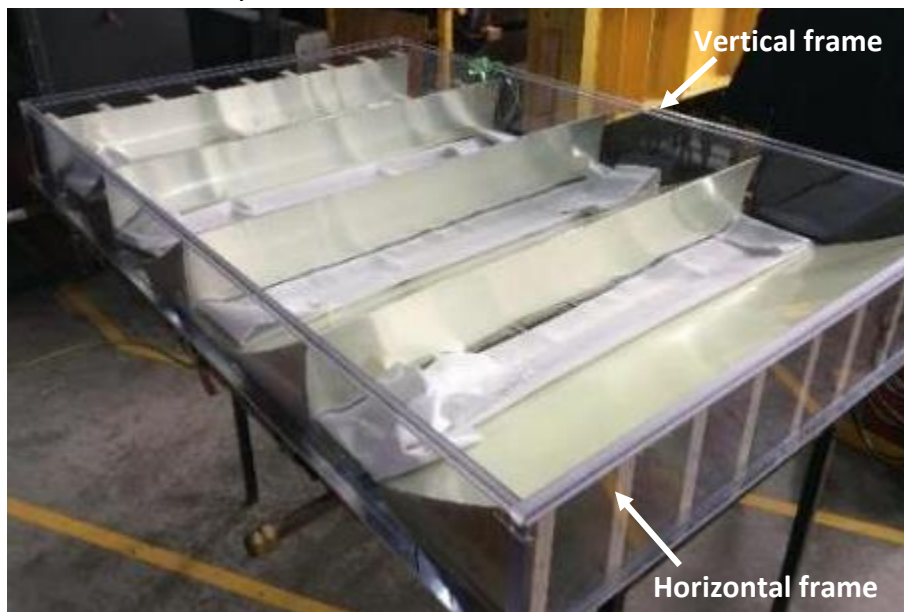
Figure 6. 17 Frame installed in the CPC System
