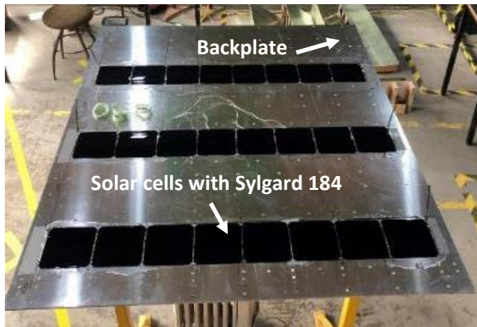
Figure 6. 26 Solar cell encapsulation process and CPC system with solar cells encapsulated
