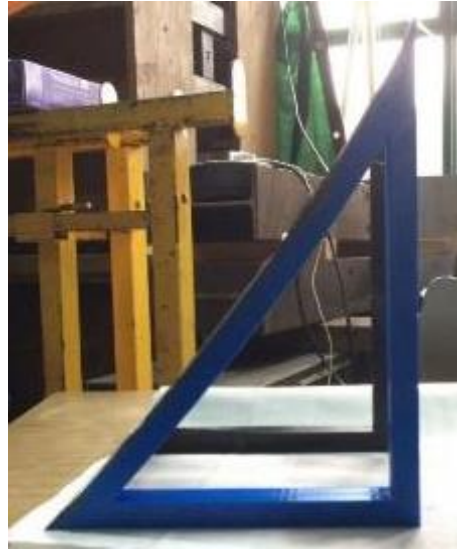
Figure 5. 4 A 3D printed Top reflector for Ferrara prototype
