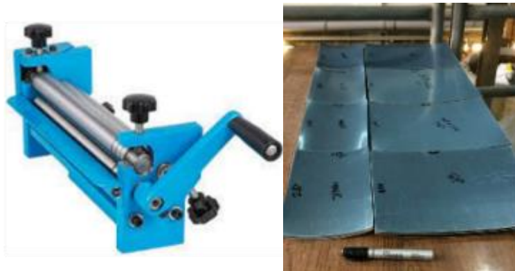
Figure 5. 8 Roller used for parabolic shape and parabolic bent pieces
