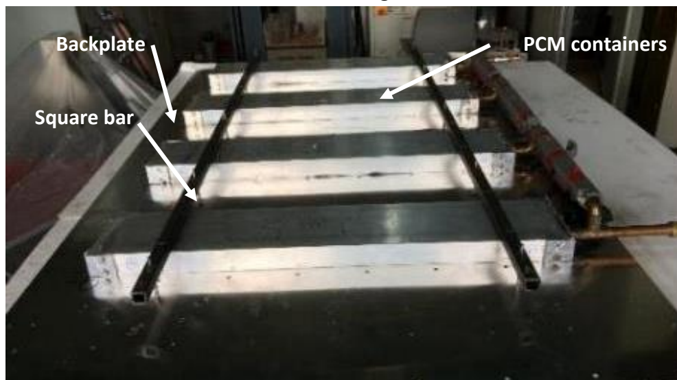
Figure 6. 19 PCM containers installed in the backplate
