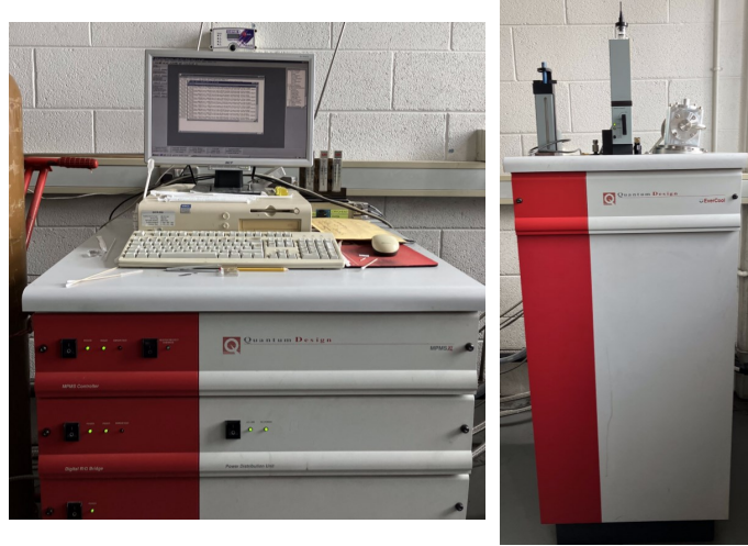
Figure 2.14: The Quantum Design MPMS-XL5 is a versatile machine used for conducting magnetometry measurements. It offers a wide temperature range from 1.8 K to 700 K, and is capable of generating a magnetic field up to 5 T. The sample is loaded into the sample space, which is located in the center of the system, as shown in the figure on the right. The PC is utilized to control and record data, as depicted in the figure on the left.
