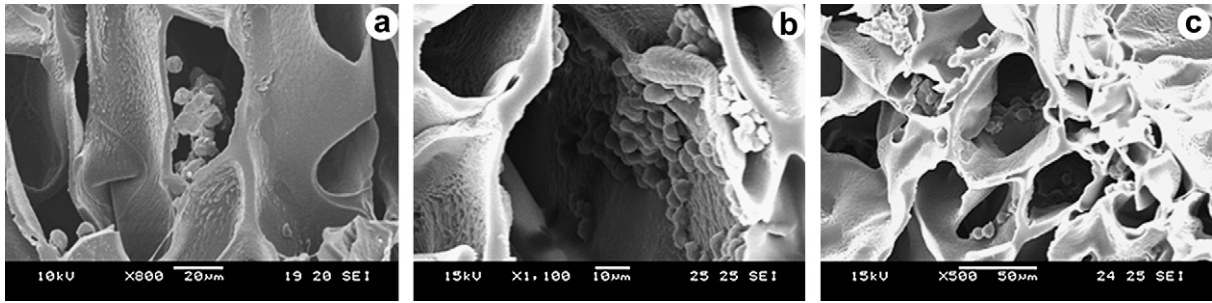
Fig. 7. Scanning electron micrographs of PU scaffolds coated with ECM proteins. Panel (a) shows the PU scaffold coated with 25 µg/ml fibronectin cultured with the Kasumi-6 cells at day 2 of culture. The cells have penetrated the pores of the scaffold and cell aggregates can be seen. Panel (b) shows the PU scaffold coated with 125 µg/ml collagen cultured with the HL-60 cells at week 4 of cultures. Colonies of cells can be seen deep within the pores of the inner section of the scaffold. Panel (c) shows the PU scaffold coated with 50 µg/ml fibronectin cultured with the K-562 cells at week 4 of culture. Cell growth appears extensive with the pores of the scaffold being occupied.
