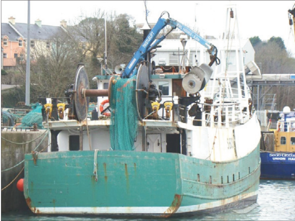
Aquila stern view showing net drum, net handling crane and Gilson frame over the bag hatch for lifting in cod end.
