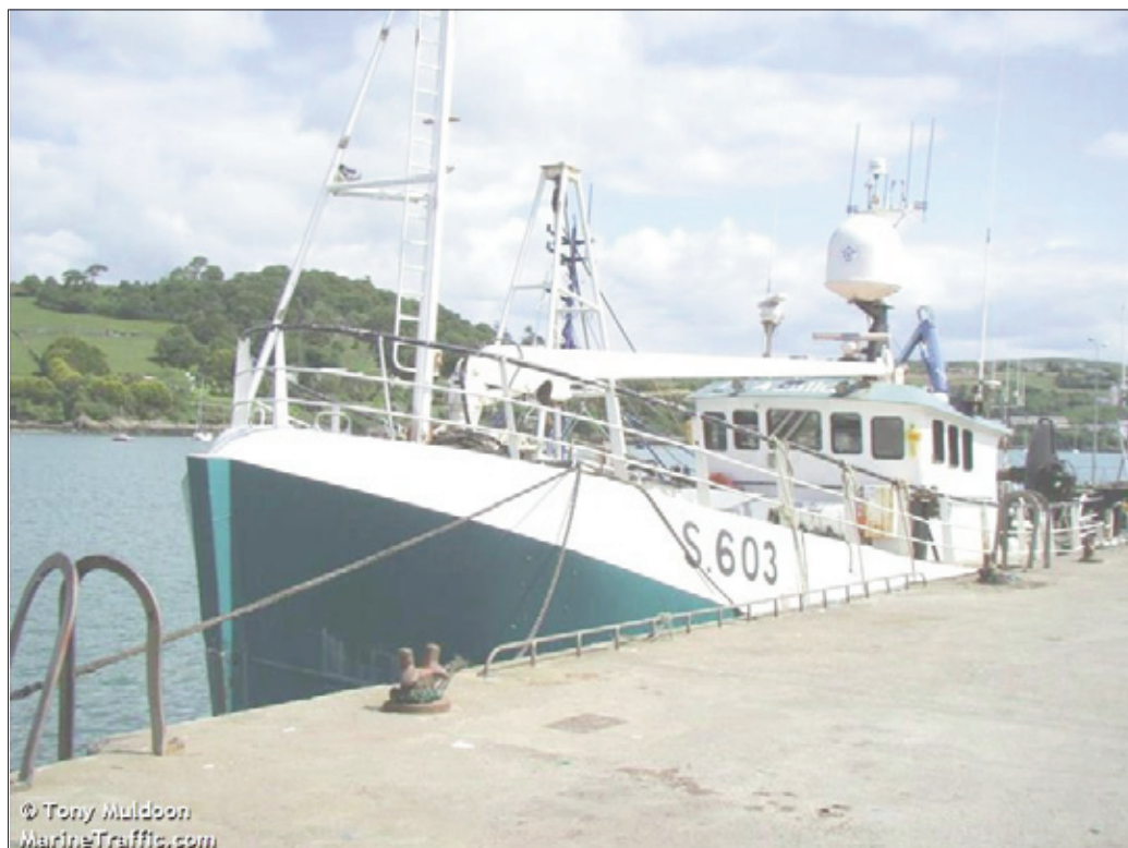
Photograph showing Gilson frame, starboard side, for lifting in the cod end and centre line deck crane for unloading catch.
