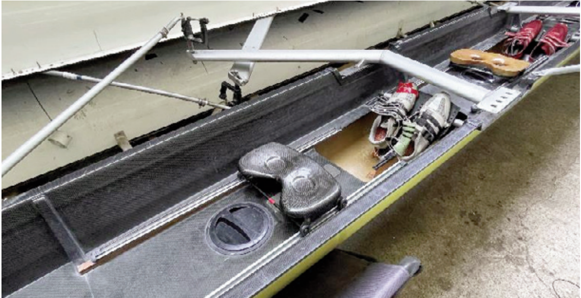
Figure 21: Example of the seating position in a competitive rowing boat, configured for sweep rowing (with only a single oar per rower).
