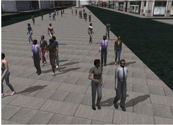
Figure 5: Virtual humans walking in groups using cohesion, separation and alignment steering behaviours.
