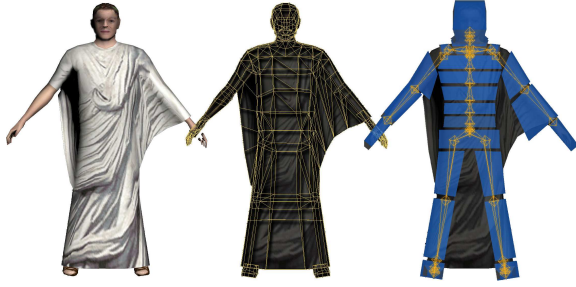
Figure 7: Textured model (left), triangle outlines (middle), underlying skeleton as oriented bounding boxes (right).
