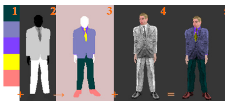
Figure 2: Billboard variety coloring steps from left to right: acquiring the modification colors (1), selecting which area to modulate using the alpha channel (2), adding the diffuse color (4) and the result in (5), from Maupe [Mau05].
