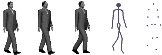
Figure 7: High resolution, low resolution, impostor, stick figure and point light source model.
