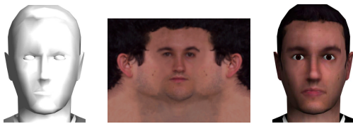
Figure 1: Simple Texturing-Mapping: (a) Mesh without texture-mapping, (b) Texture Map (c) Texture-mapped mesh.
