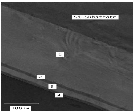
Fig. 3 Bright Field C2971 TEM image, with 5 distinct layers: Silicon Substrate, (1) 200nm SiGe layer, Ge 40%, (2) 9nm Strained Si, (3)20nm SiGe (40%), (4) 5nm Si cap.
