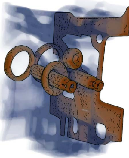
Figure 10: Two avenues of research we are investigating, line enhancements for the surrounding volume and multi-dimensional transfer functions. The first image shows an engine block with the target isosurface highlighted using Difference of Gaussian edges and the surrounding volume enhanced using suggestive contours. The second image shows the target isosurface highlighted using suggestive contours and the Kuwahara filter while also using a multi-dimensional transfer function.
