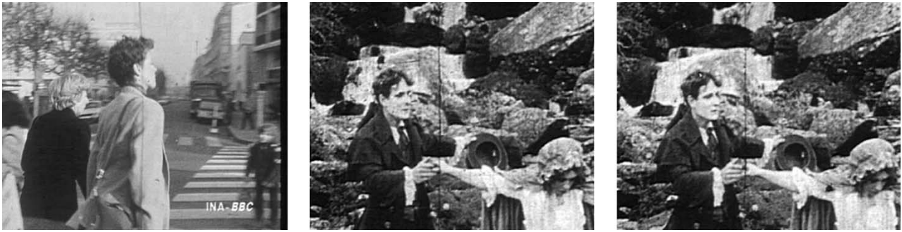
Fig. 10. Line Scratches manifest in much archived footage. They also occurs due to accidents in film developing. The color of the scratch depends on which side of the film layer it occurs. It is often the case that not all the image information inside the scratch is lost. They are a challenge to remove because they persist in the same location from frame to frame.
