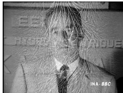
Fig. 7. Vinegar Syndrome often results in a catastrophic breakdown of the film emulsion. This example shows long strands of missing data over the frame.
