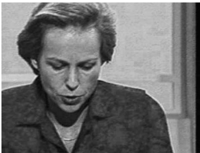
Fig. 8. Echoes and Overshoots manifest as image shadows slightly displaced from each object in the frame. When the effect is severe it is called Echo and when it is just limited to edges it is called Overshoot, as in this case.
