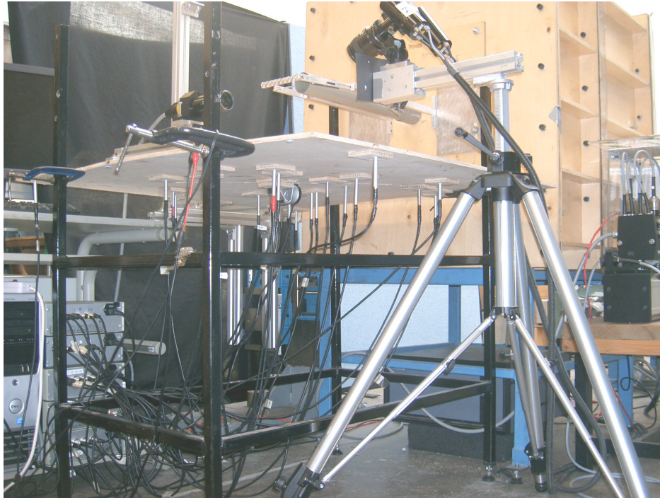
Figure 8. Planar array located below the measured volume
