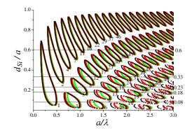
Figure 4. Maps of the photonic band-gap areas of a 1D PC comprising a periodic Si-Air structure with m = 4, calculated for normal incidence of light ( $\Delta \varphi = 0$ , black line) and for p-polarized beams with focusing parameters of  $\Delta \varphi = 5 \div 20^{\circ}$  (red line) and  $\Delta \varphi = 10 \div 30^{\circ}$  (green line). The horizontal dashed lines crosses the SB areas of PCs with specific filling fractions, for example  $f_{Si} = 0.23$  for  $\lambda/4$ -layers.
