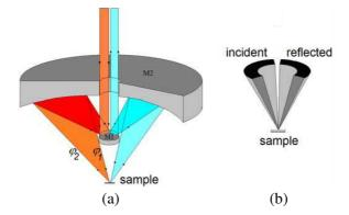
Figure 2. (a) Schematic of the beam path in IR microscope, showing mirrors M1 and M2 during measurements of reflection spectra R; (b) Shape of incident and reflected light, as truncated semi-cone volumes.
