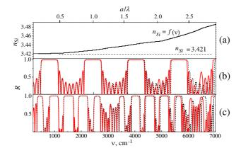
**Figure 6.** (a) Dispersion of the refractive index  $n_{Si}(\nu)$  from Ref. [14] and the reflection spectra, R calculated with (red thin line) and without (black dotted line) dispersion of  $n_{Si}$  for a 1D PC based on a Si-Air structure. The lattice constant,  $a = 4 \,\mu\text{m}$ , and the number of periods, m = 6. The filling fraction, (b)  $f_{Si} = 0.23$  and (c) 0.6 at normal incidence of light.
