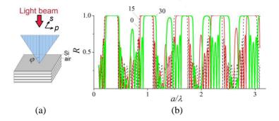
**Figure 1.** (a) Schematic diagram showing light reflection from a 1D PC (layered structure) based on "Si-Air", with number of periods, m = 4, for calculation of reflection and transmission spectra; (b) Reflection spectra (in *p*-polarisation) for a specific angle of light incidence  $\varphi$ , shown by the numbers beside the curves in degrees.
