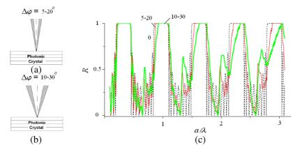
**Figure 3.** Model of focused beam in the range  $\Delta \varphi = (a) 5 \div 20^{\circ}$ , (b)  $10 \div 30^{\circ}$ ; (c) *p*-polarized average spectrum  $R_{\Delta \varphi}(\lambda)$  calculated using models in Figs. 3(a) and 3(b). The numbers beside the spectra correspond to the range of angles  $\Delta \varphi$  in degrees.
