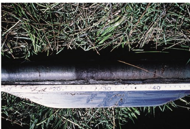
Figure 5. a) Lithostratigraphic data is commonly collected in the field using hand-corers. Here, a narrow-bore gouge auger is being used to investigate sediments in an Indonesian mangrove © Photograph, B.P. Horton; b) The altitude of sediment samples and boreholes must be measured, and their vertical relationship to tide level established. Here a total station is being used to level samples from inter-tidal flats in Indonesia © Photograph, B.P. Horton; c) Salt-marsh sediments recovered in a Russian-type corer are described in the field before being removed for laboratory analysis. In this section, bands of dark peat alternate with pale silty clay. © Photograph, R.J. Edwards.
