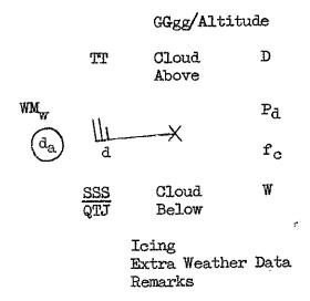
2. The various elements in the aircraft position and weather report are plotted as follows:
