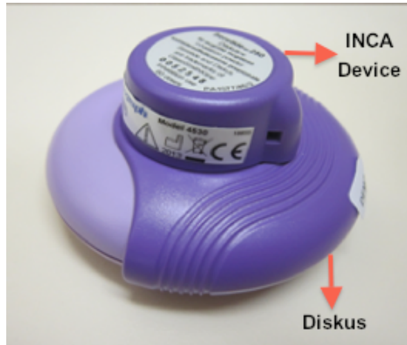
Figure 1: INCA Device and functional position on Diskus™ Inhaler
