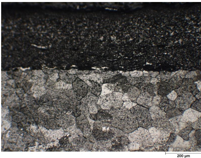
Figure 2(b): Substrate (Molybdenum) Micro-structure
