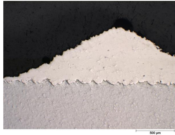
Figure 3: Typical Stellite-6 coating track cross-section on steel by SLD.
