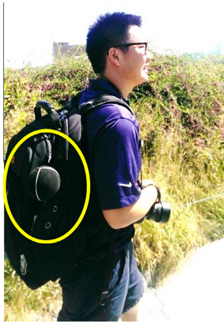
Fig. 4. Sound level meter positioned in side pocket of backpack with microphone exposed.
