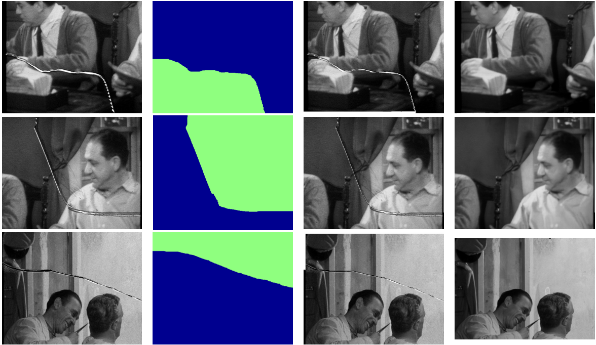
Figure 6.38: First Column (from left): Close-up of torn frames; Second Column: Close-up of the segmentation; Third: The torn frame with compensated displacement. The edges should now correctly align across the tear boundary; Fourth: The fully restored frame after missing data treatment. The missing data treatment algorithm used [60] also acts as a noise reducer.
