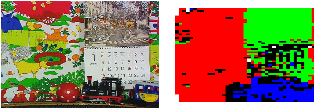
Figure B.3: This figures shows an example of the segmentation algorithm applied to a frame (shown on the left) from the “mobile and calender” sequence. In this sequence the global motion comes from a camera pan to left. The calender in this sequence is undergoing local motion (moving downwards) and the train and ball is also undergoing local motion. The image on the right shows the results of the motion based segmentation. The red segment corresponds to the motion of the background and the other colours correspond to the various local motions.
