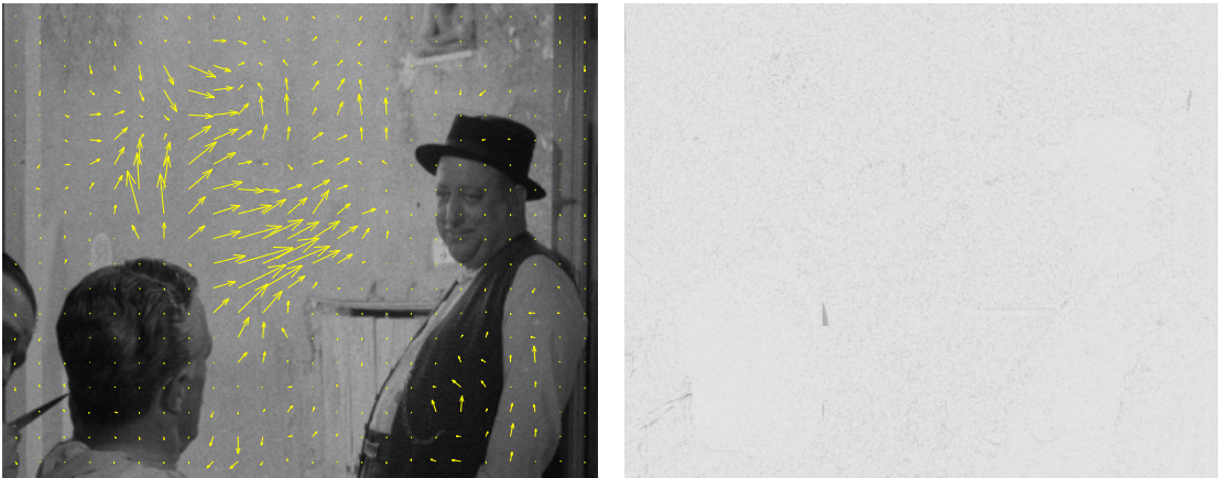
Figure 2.6: This figure shows that motion estimation failures due to ill-conditioning do not normally result in temporal discontinuities. The arrows in the left image indicate the motion of each image block. The image blocks in the flat region in the middle of the image are ill-conditioned and the vector field in this region contains large motion vectors even though this region is not moving. In the DFD for the left frame (right image), there is no temporal discontinuity in this region. Although the vectors are clearly wrong, they still match with a similar block in the reference frame.
