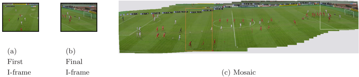
Figure 5.17: Mosaic built on a soccer sequence : Initially the camera pans left from the centre circle before panning right revealing the entire pitch. The white box shows the position of the last frame in the mosaic. The hybrid algorithm estimates the global motion accurately for most frames. However the orange box indicates an error in the mosaic caused by failure of the hybrid algorithm. This results in the remaining frames placed in the mosaic being tilted slightly upwards. See Fig. 5.18 for a more detailed description of the error.
