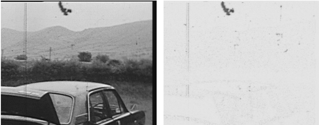
Figure 2.5: This figure demonstrates that blotches cause temporal discontinuities. The right image shows the DFD between the frame depicted in left image and the previous frame in the sequence. The dark region in the DFD indicates high values caused by the blotch. High DFD values correspond to temporal discontinuities in the image sequence.
