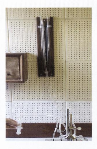
Figure 3. Photograph of the Pressure calibration system for PERCI SARS indicating the U tube manometer, syringe attached to the pressure transducers.
