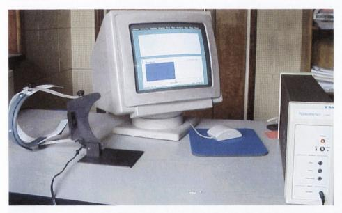
Figure 1 Photograph of calibration set up for Nasometer, indicating the bar mode on the computer screen.
