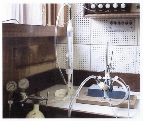
Figure 5. Photograph of the Airflow calibration set up for PERCI SARS, indicating the airtank, meters, rotameter and tube attachment for pneumotachograph.
