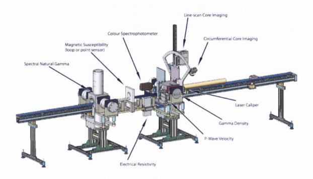
Figure 3.18: 3D diagram of the MSCL-S (taken from www.geotek.co.uk).
