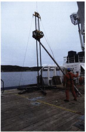
Figure 3.14: The Geocorer 6000 set up for coring on the ILV Granuaile.
