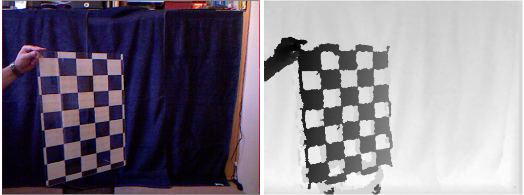
Figure A.4: The glass chessboard used to calibrate the Kinect Camera, both the colour and the depth sensor can see the pattern.
