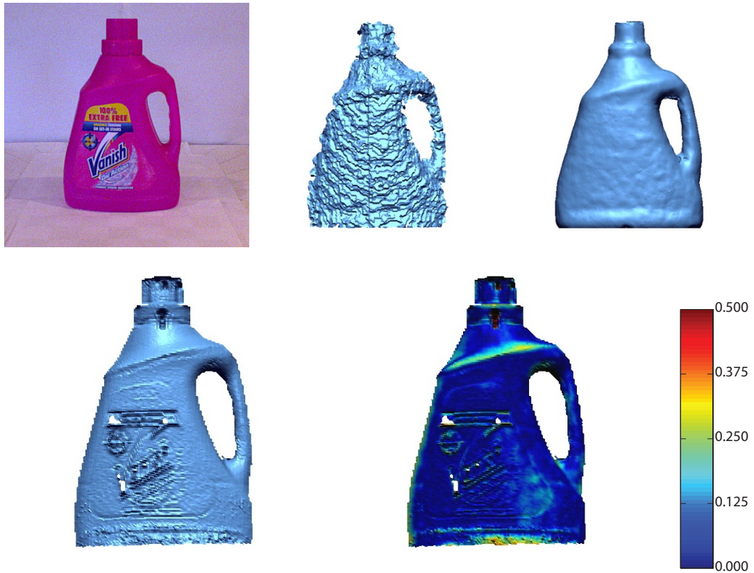
Figure 5.22: Comparison between reconstruction method and laser scan. The top left image shows an image of the object, the top middle image shows the raw data from the Kinect camera, the top right image shows the reconstruction of the object. The bottom left image shows the raw data from the laser scan of the object and the bottom right image shows the error between the reconstruction and the laser scan. The error bar scale is 0-0.5 cm and the object is 18 \times 10 \times 27 cm. The average error is 0.765 mm.
