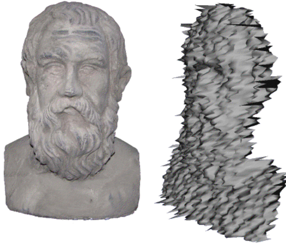
Figure 2.4: The right image gives an example of the raw data from a time-of-flight depth camera of the object on the left as presented in [20]
