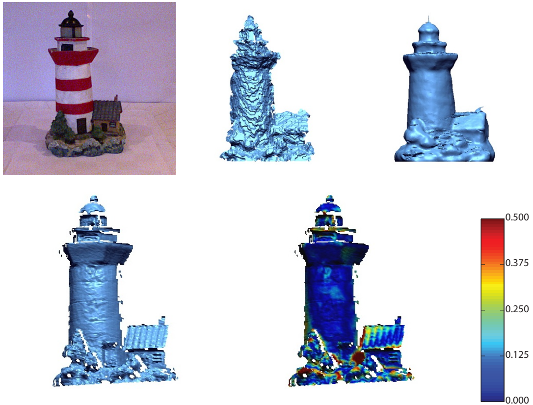
Figure 5.21: Comparison between reconstruction method and laser scan. The top left image shows an image of the object, the top middle image shows the raw data from the Kinect camera, the top right image shows the reconstruction of the object. The bottom left image shows the raw data from the laser scan of the object and the bottom right image shows the error between the reconstruction and the laser scan. The error bar scale is 0-0.5 cm and the object is 18 \times 16 \times 26 cm. The average error is 1.4 mm.
